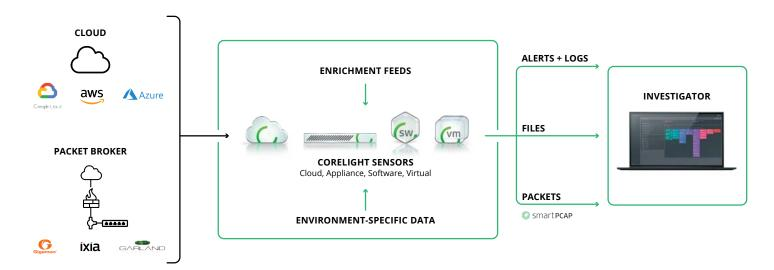
Corelight alerts and evidence stream from deployed sensors to Investigator for triage and incident response. Investigator also exports to a number of SIEM and XDR solutions.
