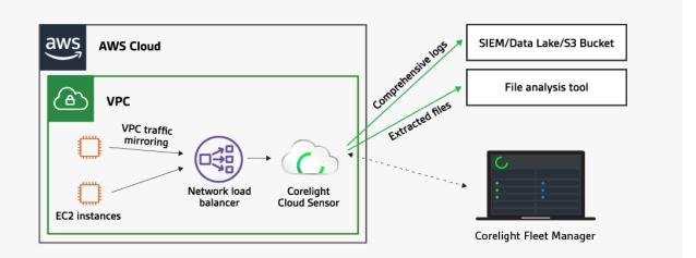
The Corelight Cloud Sensor can ingest traffic via Amazon VPC traffic mirroring (enabled per EC2 instance) or via an Amazon Network Load Balancer, streaming logs and extracted files to SIEMs, Amazon S3, or file analysis tools. Customers can fork and filter the data via Corelight's management console and easily manage multi-sensor environments with Corelight Fleet Manager's sensor policy templates and role-based access controls.
